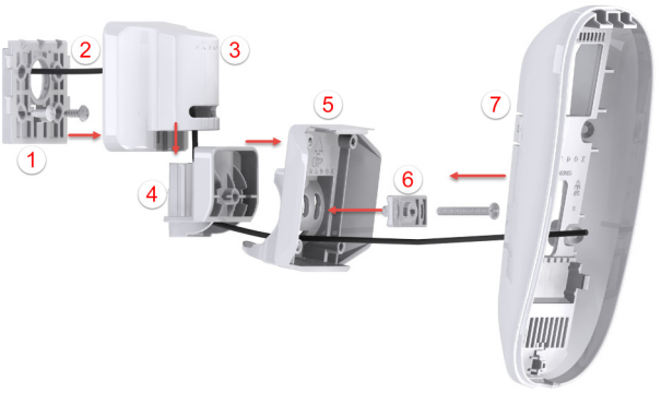
Figure 4 – Mounting HD77 Camera with Swivel Brackets
